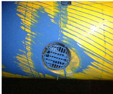
Fig Paint test result of a LNGC with bow thruster(tunnel with scallop, grid and CPP)
